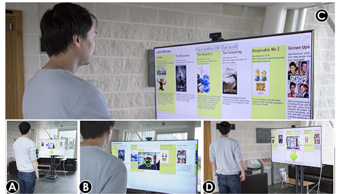
Figure 1. GazeHorizon enables passers-by to interact with public displays by gaze. The system detects users walking up to a display (A), provides interactive guidance to bootstrap use of gaze (B) and lets users navigate displayed information using horizontal eye movement (C). When a user walks away, the system is immediately ready for the next user (D).
