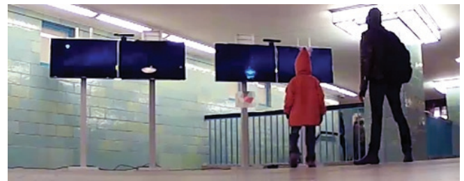
Figure 7. Two screen pairs were set up in the subway station, with a Kinect mounted on top of each to track users.
