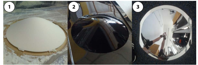
Figure 5. 1) Vacuum forming tool, 2) mirror body before and 3) after metalization
